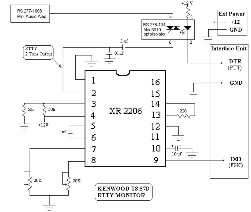
This circuit was designed to allow the monitoring of FSK rtty tones, the Kenwood 570 has a design flaw in that it has no way to monitor the rtty output in FSK mode. This circuit allowed me to monitor the rtty tones with no internal mods to the radio.
